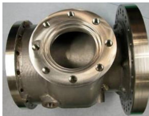
FIGURE 7 MIRA CH4 TURBINE MANIFOLD PRODUCED BY DMLS TECHNIQUES
