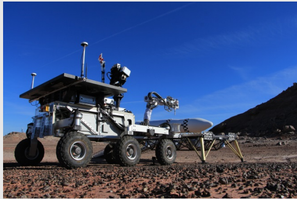
CSA Mars Exploration Science Rover (MESR) transferring a soil sample to a Mars ascent vehicle mock-up during the 2016 Mars Sample Return Analogue Deployment
