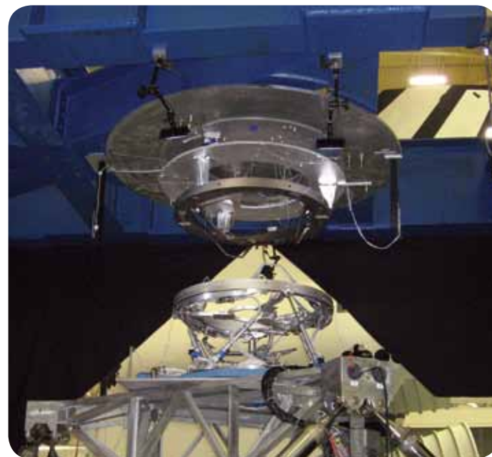
A prototype of the NASA docking system that meets International Docking System Standards requirements undergoes dynamic testing at the NASA Johnson Space Center.
