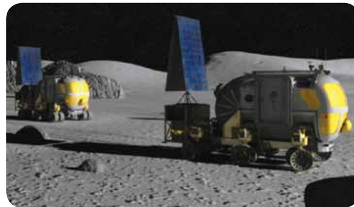
Small pressurized rovers on the moon will increase crew mobility and can be reused at different landing sites.
