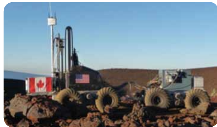
Canadian Juno Tandem Rover carrying the Regolith Environment Science Oxygen & Lunar Volatile Extraction (RESOLVE) payload and the Tridar navigation unit at Mauna Kea deployment site in 2010.
