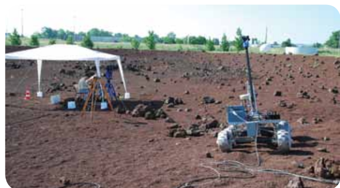
Experimental rover testing in CNES Mars-yard.
