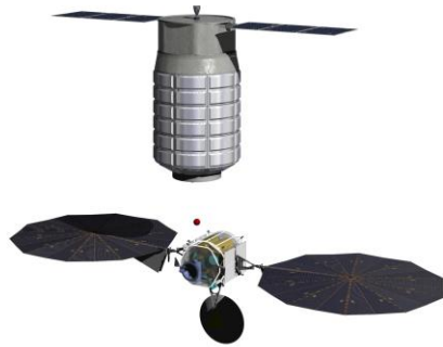
Figure 8 – Scenario 6E – Logistics Module (Conceptual Design)
