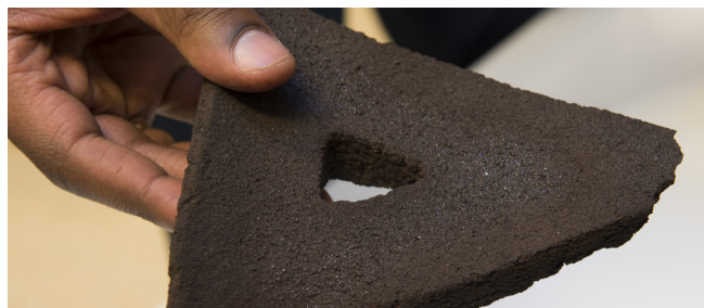
A triangular brick 3D printed out of simulated moondust using concentrated sunlight. (ESA/G. Porter)
