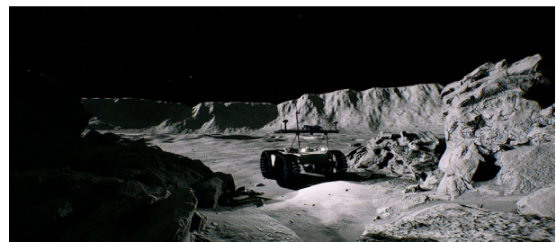
Unreal Engine rendering of the rover within the Moonscape using the scaled version of a Lunar Orbiter Laser Altimeter Digital Elevation Model. (CSA)
