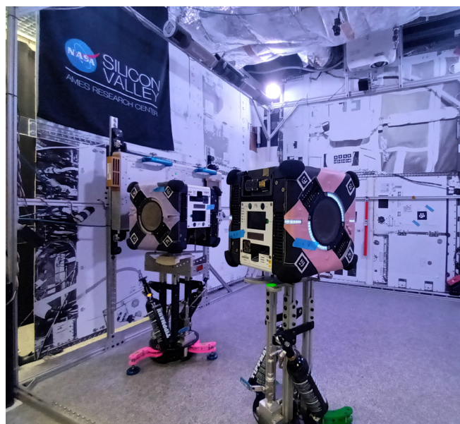
CSIRO's multi-resolution scanning payload attached to an Astrobees robot platform in a simulated ISS environment at NASA Ames Research Center. (CSIRO)
