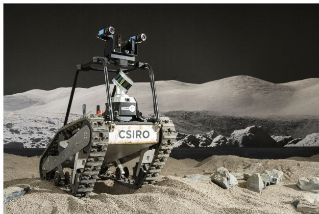
CSIRO's In-Situ Resource Utilisation Facility includes a lunar testbed that simulates some of the physical characteristics of the Moon's surface for realistic testing and evaluation of assets such as rovers and related equipment. (CSIRO)
